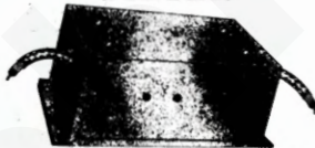
Large shielded resistor type filter unit for use in ignition system of oil burner (5000 ohms)
