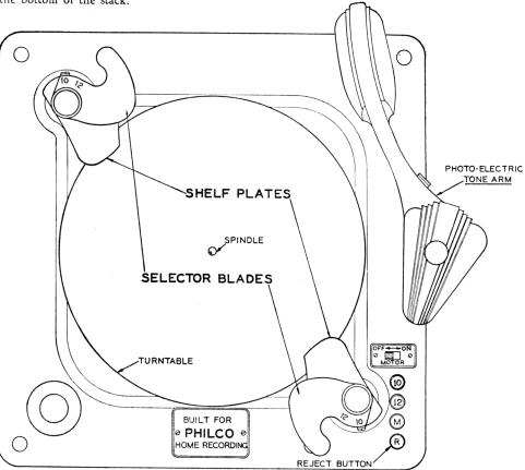
To set for record size: (1) Clasp one of the posts underneath the shelf plate, with thumb and finger of left hand. With right hand, lift knob and turn selector plate until the figure 10 or 12 (whichever size you want to play) is opposite the pointer. Do the same with the other post. Both selector plates must be in 10 or 12 position. (2) Push button marked 10 or 12, as required (see above illustration).
