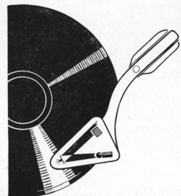
9. . . . Showing the location of the light, the mirror and the photo-electric cell in the PHILCO PHOTO-ELECTRIC REPRODUCER.
