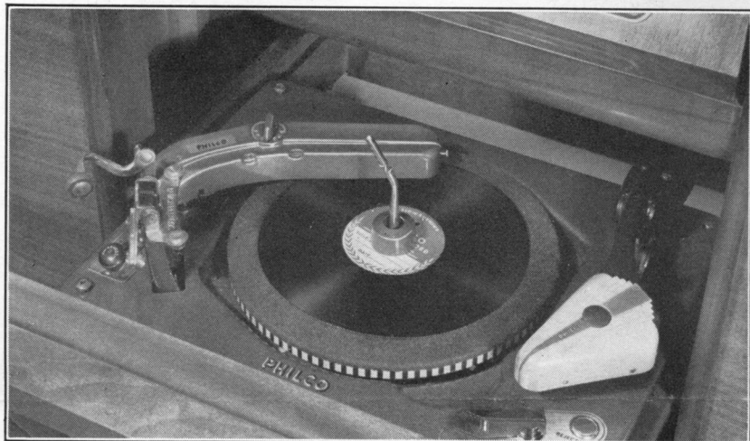
Showing Home Recorder Installed
