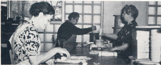
In the foreground, Charlotte Kessler rolls vinylite wires before they are dipped into molten lead. In the background, Myrtle Bellis and Eva Jewell are dipping wires.
