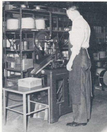
Clyde Mock is seen here operating the Flexo Press (nicknamed the spaghetti cutter). This machine cuts sleeving, which is a preparation to prevent wires from shorting. Clyde is set-up man and relief operator for this department.
