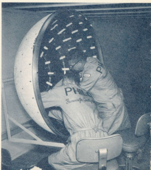
Philco laboratory technician puts finishing touches on a solar cell array module, containing 84 solar cells. A total of 228 such modules are used.
