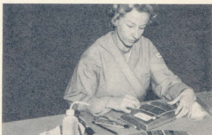
Philco laboratory technician puts finishing touches on a solar cell array module, containing 84 solar cells. A total of 228 such modules are used.
