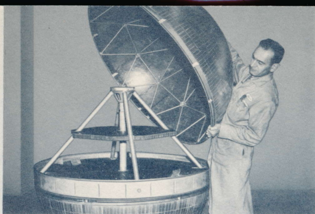
Epoxy fiberglass shells of the Courier are mounted on dummy structure to check the fit of all parts.
