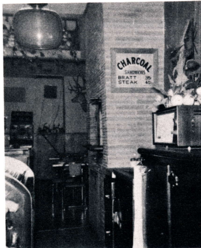
Here's an interesting variation of the same idea. The picture tube has been installed upside-down, with the base screwed into the ceiling, eliminating the need for a shelf. The picture was reversed so that it is viewed right side up. Installation was by William Ott, Ott Hardware Company, Baraboo, Wis.
