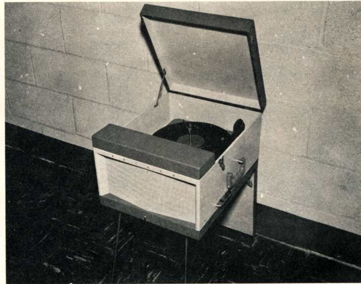
Twin speakers are featured in this new Philco "Miss America" portable, automatic 3-speed phonograph. For more portability, it has wrought iron legs which fold into the cabinet making easy conversion from table to console model.
