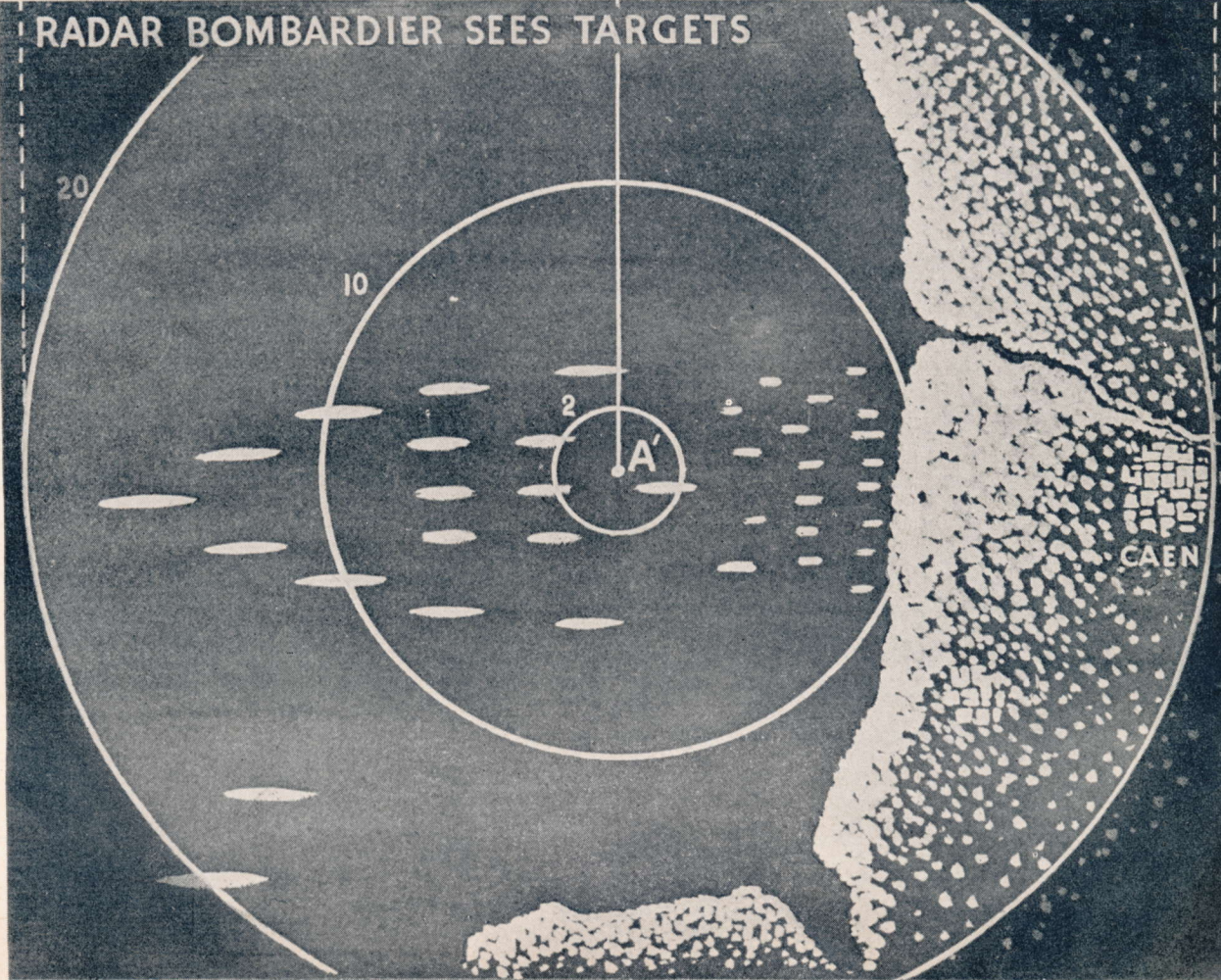
Diagram showing what the Philco Radar Bombsight ("Mickey") does.
