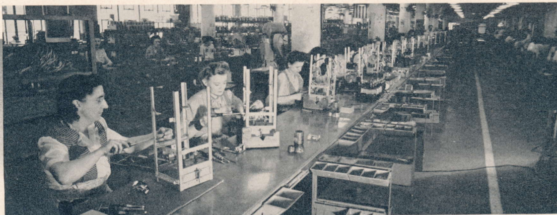
Philco high-speed assembly line for radar transmitters.
