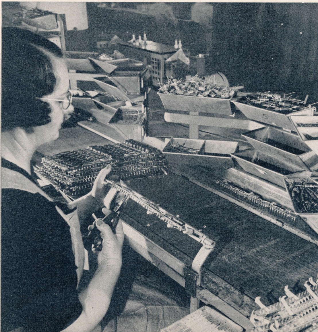
Special jig speeded Philco production of radar sub-assemblies.
