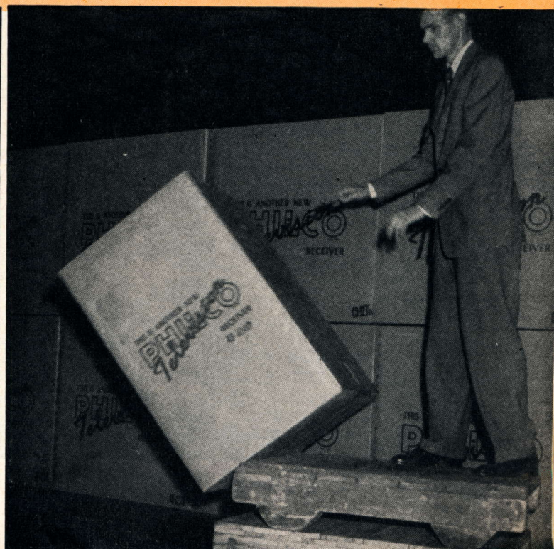
Drop tests performed on new and completely packed TV receivers, simulates abuse instrument may receive in shipment
