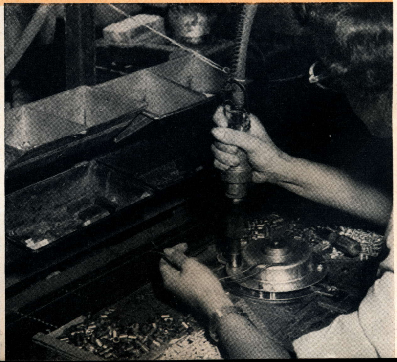
After connecting leads have been soldered to the start and finish of focus coil windings, unit is assembled into metal housing as shown
