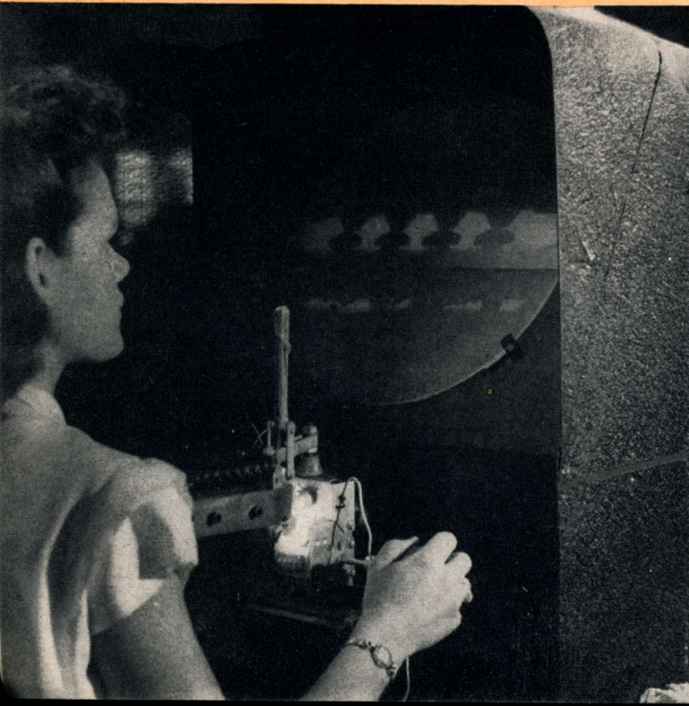
Production type comparator test equipment checks RF turret tuner switch contacts before mounting sub-assembly on receiver chassis
