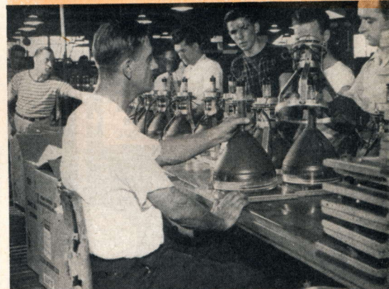
TV components that are sub-assemblies are constructed on auxiliary production lines Riveting tube sockets and terminal strips onto the main chassis is primary operation
