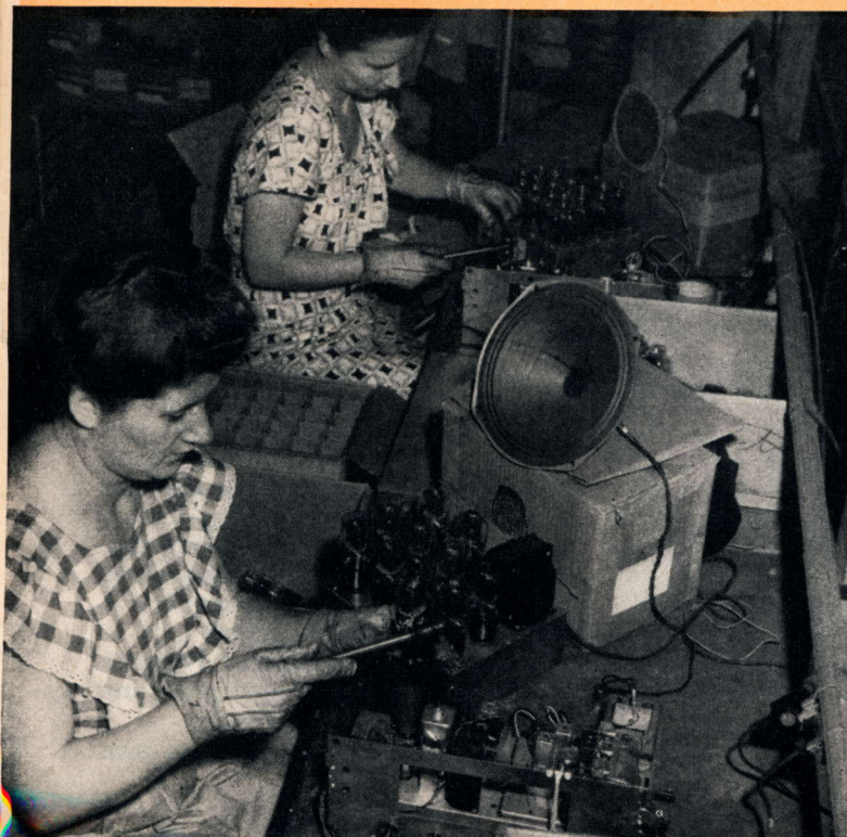
New tubes undergo an actual operation test in radio receiver chassis before they are released as production components
