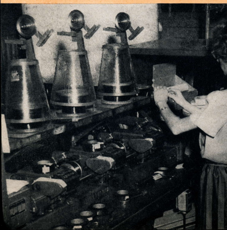
Three cathode ray tube focusing coils being wound simultaneously. Machine stops automatically when required turns are wound
