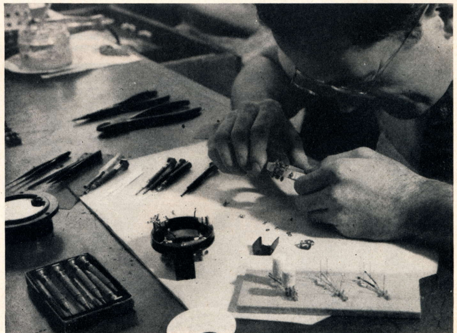
A complete stock of spare parts for all basic meter movements used is maintained so that necessary repairs can be effected promptly. Note jig for holding pointers, bottom right
