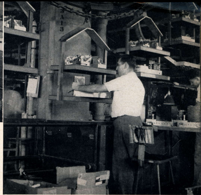
After alignment, chassis are loaded on a monorail conveyor that transports them to second floor for cabinet mounting
