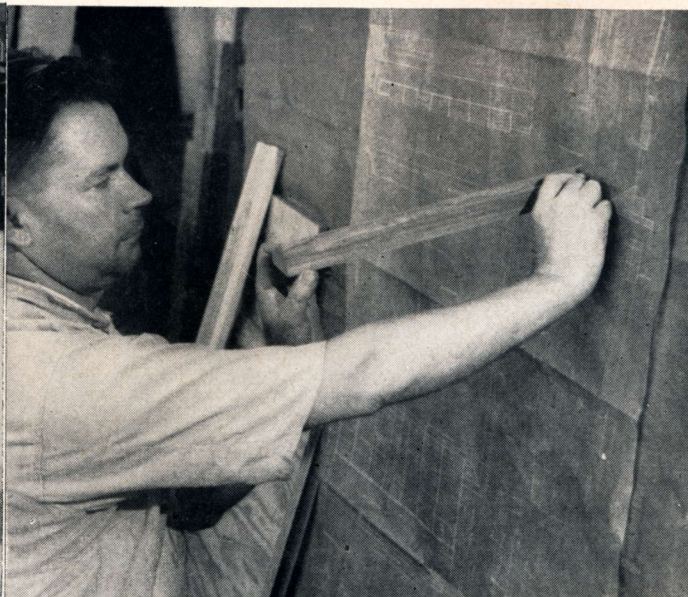
Cabinet-makers check the size of each component part against full-scale drawing and use production types of woodworking machinery
