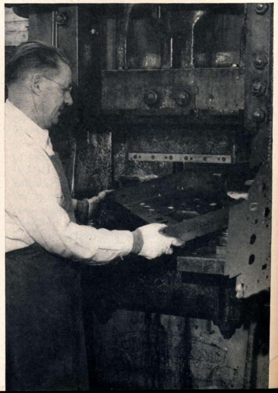
Bending sides, inserting reinforcing indents, makes punched blank semi-rigid structure
