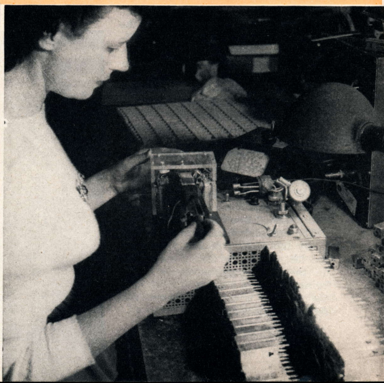
Incoming shipment of IF transformers for TV receivers being checked for frequency response and output by correctly pre-tuning each unit
