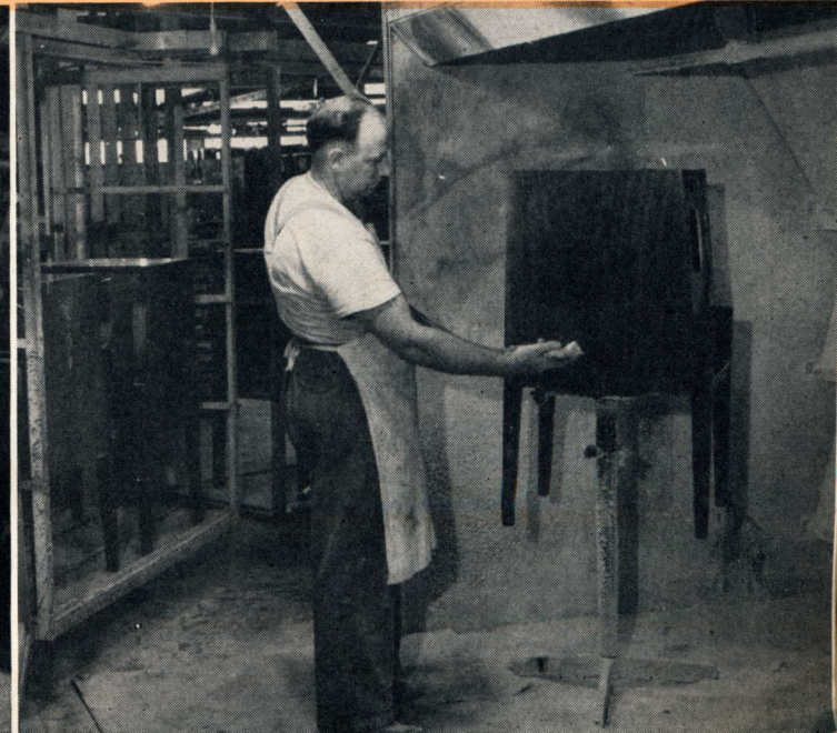
Consolette cabinets are carried by monorail conveyor to a specially designed spray booth where a final lacquering operation is performed
