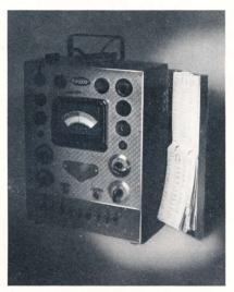
it is a simple matter for him to insert the new cards on the protected metal loose-leaf binder at the side of the Philco Model 7050 tube tester. This device enables owners of the Philco Tube Tester to keep their instrument up to date at all times
