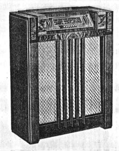
340 xx Eight tubes. Six Electric Push-Buttons. Inclined Sounding Board, Inclined Control Panel, Philco Disc Controls for tuning of all stations, Cathedral Speaker. Handsome cabinet of Walnut. Tuning ranges cover Standard Broadcasts, Day and Night Foreign and Domestic Short-Wave, Police Calls, Ships and Amateurs \$149.50
