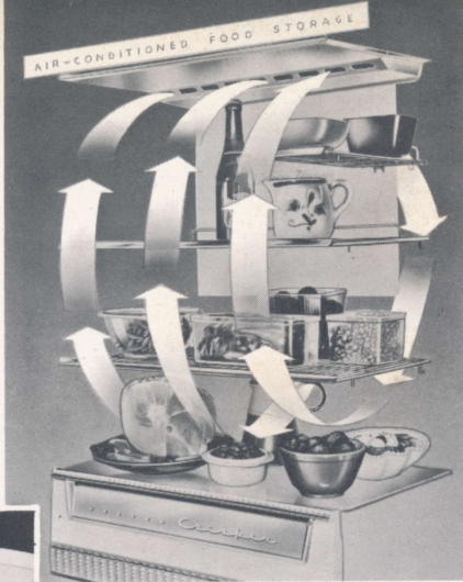
Diagram above shows air entering grille to be cooled and dehumidified.
