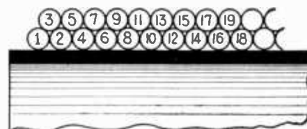
Method of bank winding wire on a coil form.
