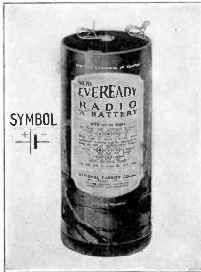
Fig. 3. A dry cell "A" battery
