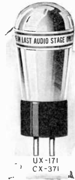
A new storage-battery type power amplifier tube, for use in the last stage audio amplifier only. This tube takes the same filament voltage and filament current as the No. 112 tube but employs a "B" voltage of 180 and 40½-volt "C" battery. Special means should be provided for handling its heavy output.
