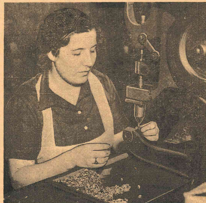
EYELET MACHINE , operated by Jane Ciesielska (Department 41) is equipped with a steel sleeve around the plunger. Sleeves close to the work and does not permit operator's fingers underneath the punch. This device is an example of the ceaseless efforts to promote safety. Jane is co-operating by wearing a hair net, to prevent her hair catching in machinery.
