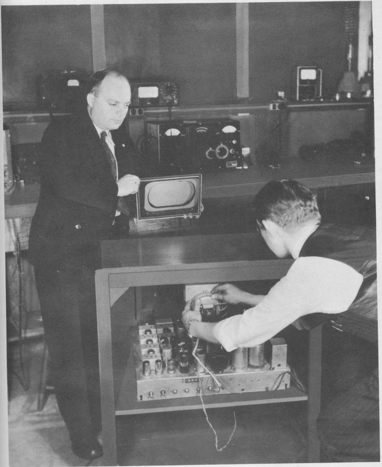
Figure 52. Use of Mirror in Making Rear-Chassis Adjustments.
