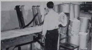
The insulation cutting board.
