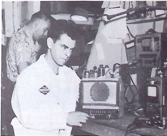
Richard Hajian tests a tube while making an auto radio repair. Regardless of the reason the radio was brought in, a complete check is made of the entire radio before it is returned to the customer.
