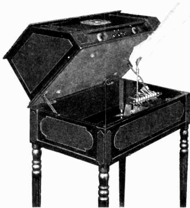
Figure 5—Installing condenser bank of A.C. Package UP-972
