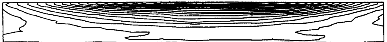
FIGURE 6: Thermographic image in the SAR plane. E field parallel to the cut.
