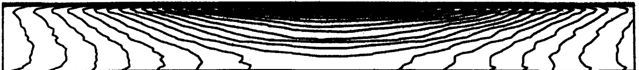
FIGURE 5: Thermographic image in the SAR plane. E field normal to the cut.
